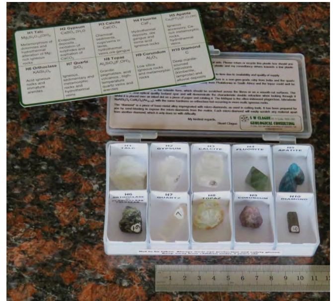
Figure 2 – Boxed set of Mohs Hardness testing minerals, with glossy information card insert.
