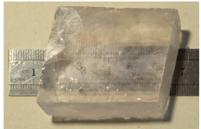
Figure 1 – Calcite CaCO 3 , Iceland Spar variety, showing double refraction of the ruler through the cleavage rhomb.
