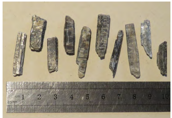
Figure 7 – Kyanite Al_2SiO_5 , as bladed, triclinic crystals.
