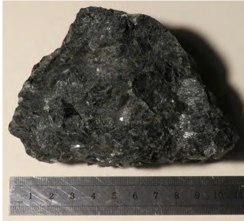
Figure 4 – Hornblende: Ca_2(Fe^{2+}, Al)(AlSi_7O_{22})(OH)_2 (Norway), in a monoclinic crystal aggregate.
