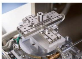
Figure 1. The Micro-XRF works with a fixed beam and cannot raster like an e-beam. Therefore, a special stage (Rapid Stage) has been developed for high-speed element distribution measurements with X-ray excitation. This stage is mounted on top of the existing SEM stage and can be easily removed when it is not required.
