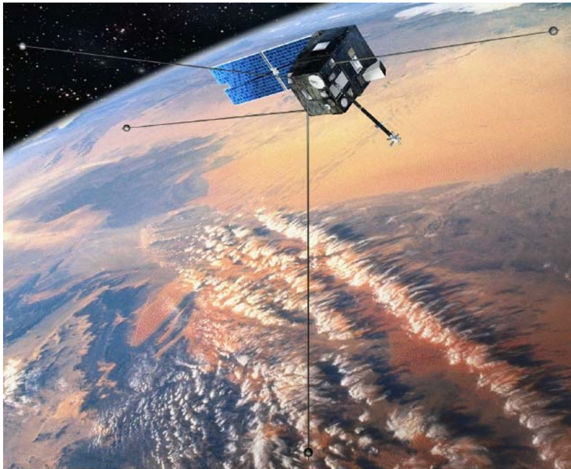
Figure 1: The micro-satellite DEMETER in flight configuration (CNES document). The dimensions are 60 x 60 x 80 cm 3 and the weight is around 130 kg. The solar panel in blue can be seen on the left. On the right there is a 1.9m boom supporting the three magnetic sensors and the Langmuir probes. There are four spheres for the electric sensors at the end of 4m booms.
