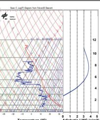
Figure 2. Temperature & Dew-point profiles measured by the Falcon (left panel). The right panel shows the calculated adiabatic LWC profile.
