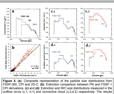
Figure 5. (a): Composite representation of the particle size distributions from FSSP-300, CPI and 2D-C. (b): Extinction comparison between PN and FSSP + CPI derivations. (c) and (d): Extinction and IWC size distributions measured in the outflow cirrus (c, d, 1) and convective cloud (c, d, 2) respectively. The results highlight a quite good consistency of microphysical parameters derivations.
