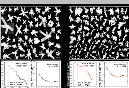
Figure 6. Examples of ice crystal images measured by the CPI. **Left panel:** Bullet-Rosettes sampled near -45°C in the outflow cirrus. **Right panel:** Chain-like aggregates observed near the top of the convective cloud (11.2 km/58°C). The corresponding particle size distributions and scattering phase functions with mean values of parameters are displayed on the bottom panel.
