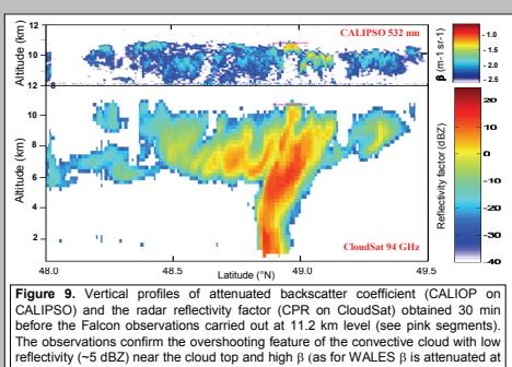
Figure 9. Vertical profiles of attenuated backscatter coefficient (CALIOP on CALIPSO) and the radar reflectivity factor (CPR on CloudSat) obtained 30 min before the Falcon observations carried out at 11.2 km level (see pink segments). The observations confirm the overshooting feature of the convective cloud with low reflectivity (~5 dBZ) near the cloud top and high β (as for WALES β is attenuated at lower altitudes indicating dense cloud with high ice particle concentration).
