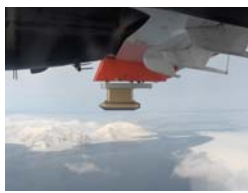
The Cloud Particle Imager (CPI) on the Do 228 (AWI) during the ASTAR experiment (Spitzberg, 2007).
