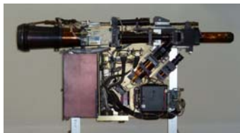
The Cloud Particle Imager (CPI) probe without canister.
