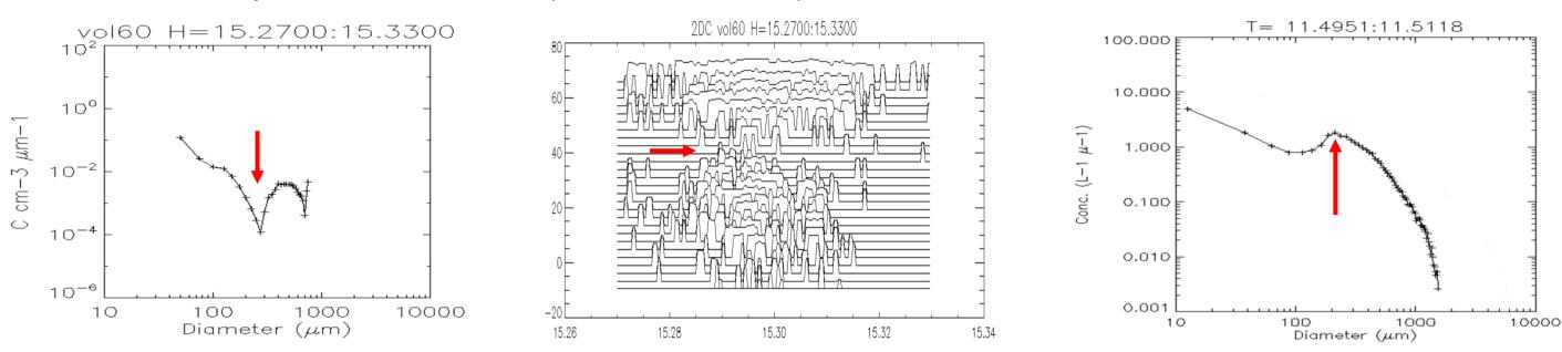
In some cases this mode of the spectrum could be interpreted as a lagrangian mixing (cloud) particles in the same place having had different histories) of different populations of hydrometeors (for example small pristine crystals and precipitating graupels).
