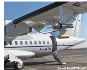
The Polar Nephelometer on the ATR-42 (Météo-France) during the POLARCAT experiment (Kiruna, 2008) with the Cloud Particle Imager (CPI) and the PMS 2D-P.
