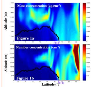
Dust mass (Figure 1a) and number (Figure 1b) concentration for the SED simulation. The black line corresponds to the top of the monsoon flux calculated from wind directions in the simulation.
